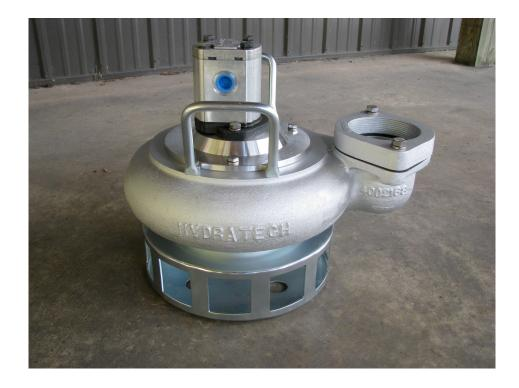
This pump is designed to operate with hydraulic <u>input flows to 10 GPM and a maximum pressure of 2800 PSI</u>. Hydraulic circuits must be open center, single direction and have an unrestricted return flow from the hydraulic motor to the oil reservoir.
